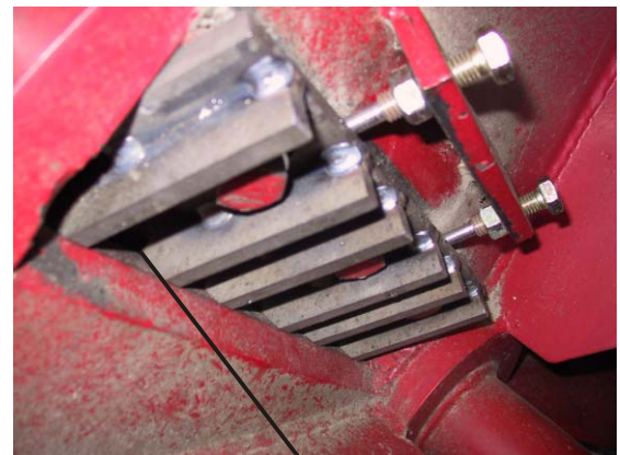
STICKKNIFE (extra) screwed on standard knife
