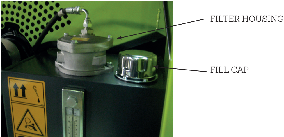
HYDRAULIC OIL TANK
