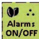
When button is pressed, hoppersensors are deactivated and yellow Alarms OFF indicator is shown on main display
