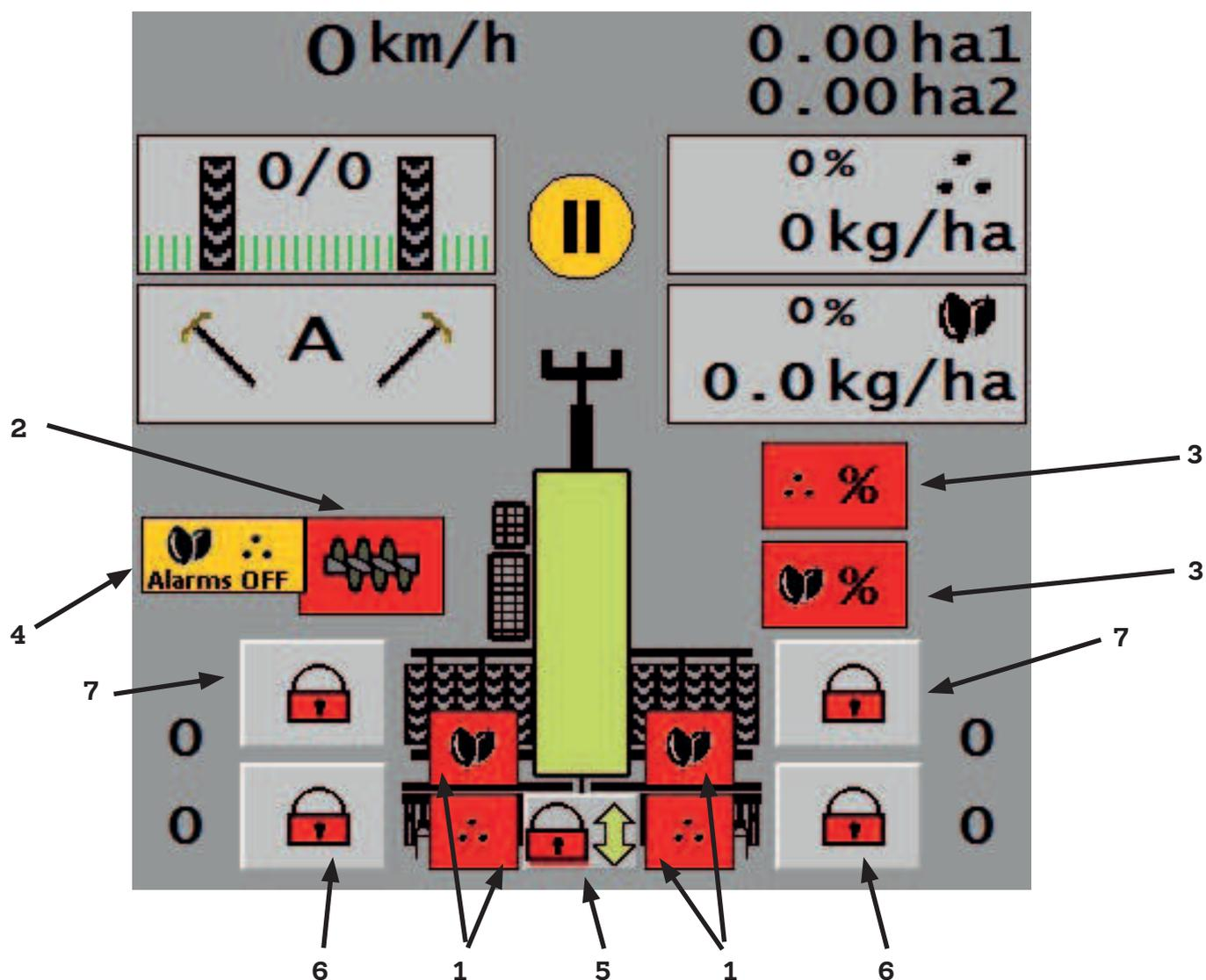
1. Wing hopper level sensors indicator lights
