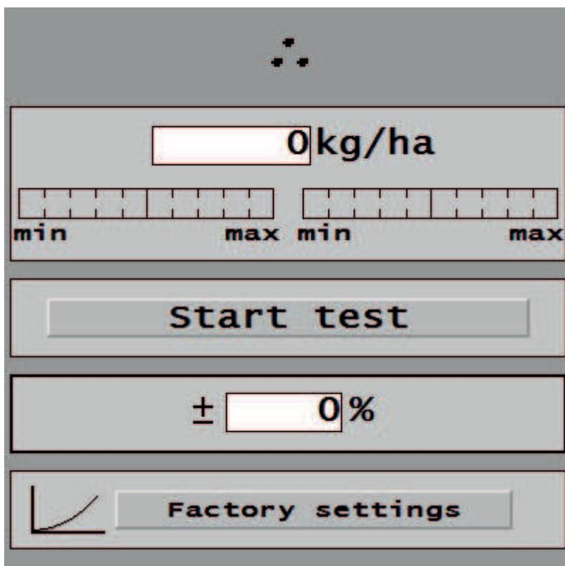
When Start test button has been pressed, page on right hand side opens. There you can give the weighing result. Calibration test is made by rotating left and right hand side fert gearboxes 10 r, which equals 100 square meters. Count left and right side weight together and give that result to kg line. Confirm result with green V button
