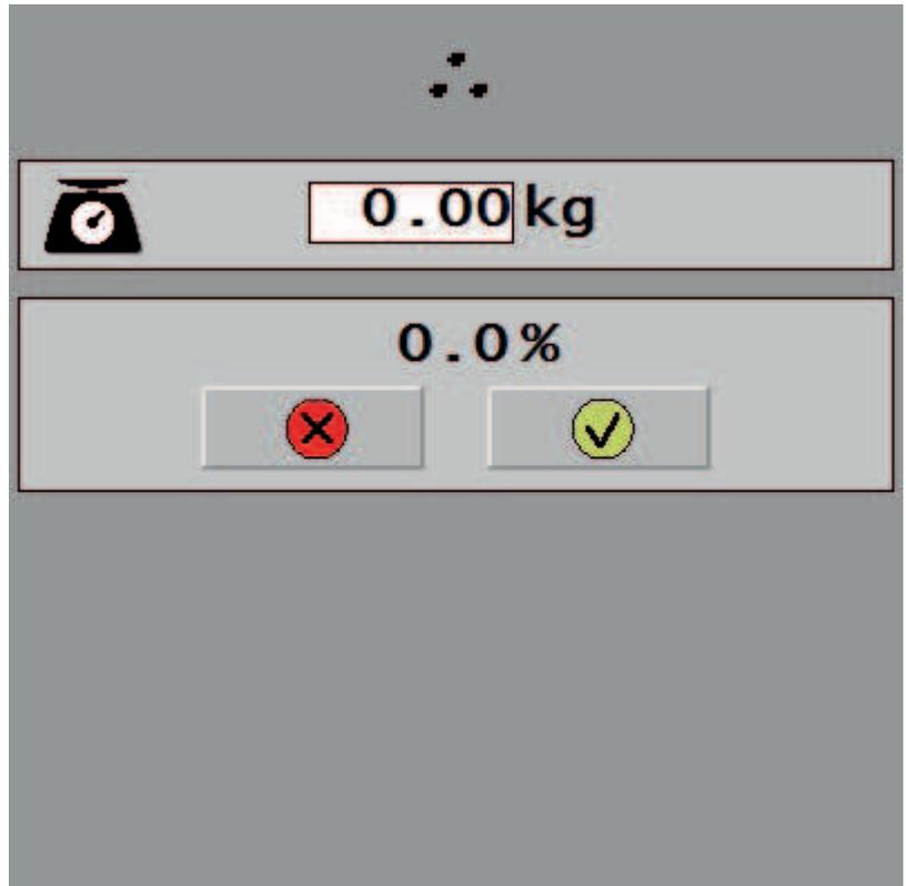
After confirming result Linak actuators are moving to place software thinks they have to be. Correction is shown as % on display. Make calibration test one or two more times so that correction % is between 0-4%.
