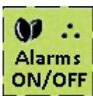
Press the Alarms button to disable the wing hopper alarms (the main screen shows the yellow “Alarms OFF” icon).
