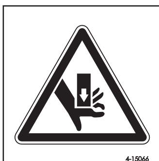
Danger of being pressed
