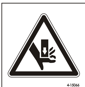
Danger of being pressed
