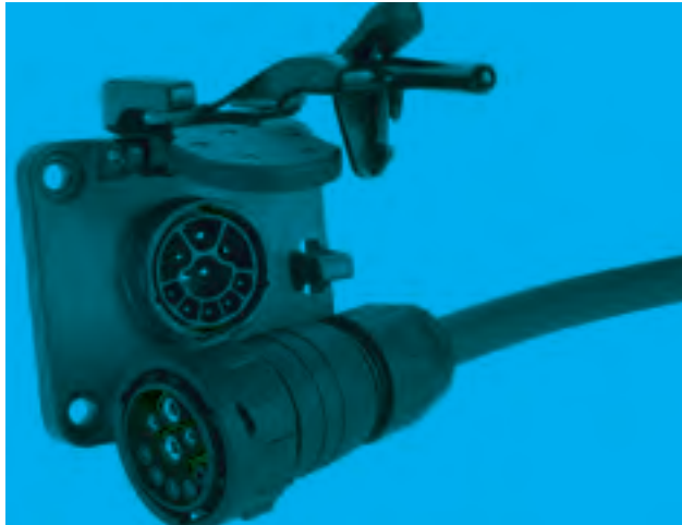
Picture 73. The ISOBUS cable of the seed drill and the plug on the tractor.
