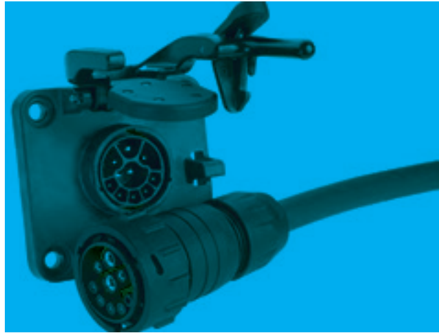
Picture 14. The ISOBUS cable of the seed drill and the plug on the tractor.
