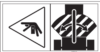
Danger of compression between the machine and traktor
