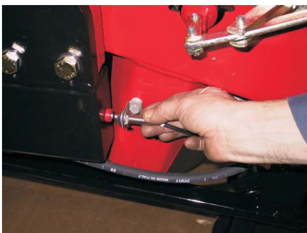
1. The sensor of lifting and lowering of the drill is placed to the right side of the machine, at the end of the bogie arm.
