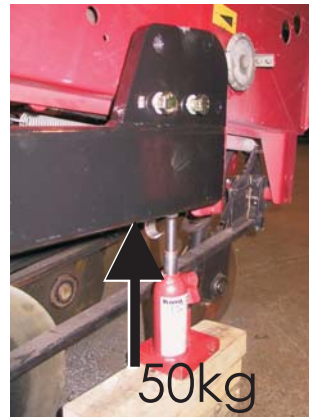
5. and 6. Support the arm with, for example, a jack, while turning it, to help locating the attachment screw holes (4 pcs). Required lifting power is 50 kg. The height adjustment screw will also take its place when the arm turns.
