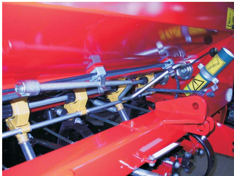
9. Placement of the calibration test lever (in front of the machine, under the fertilizer hopper).
