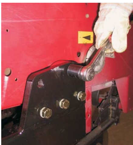
7. Tighten the arm attachment screws with care (4 pcs/side).
