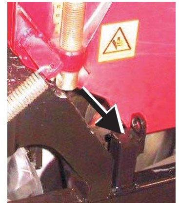
5. and 6. Support the arm with, for example, a jack, while turning it, to help locating the attachment screw holes (4 pcs). Required lifting power is 50 kg. The height adjustment screw will also take its place when the arm turns.
