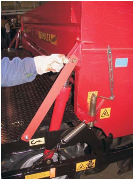
1. Detach the linchpins and remove transportation supports from between cylinder brackets and foot step frame.
