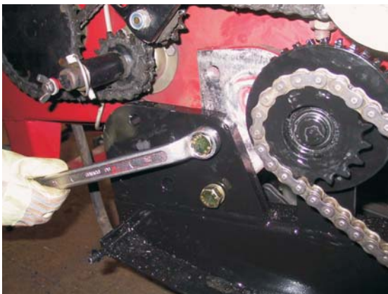
4. Remove the upper transport attachment screw from the arm to let the arm turn pivoted on the lower screw. Then the wheel assembly is also able to move to its place behind the machine.
