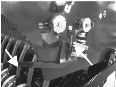
Figure 6a Hopper handle and locking system, identical on both sides of the machine
