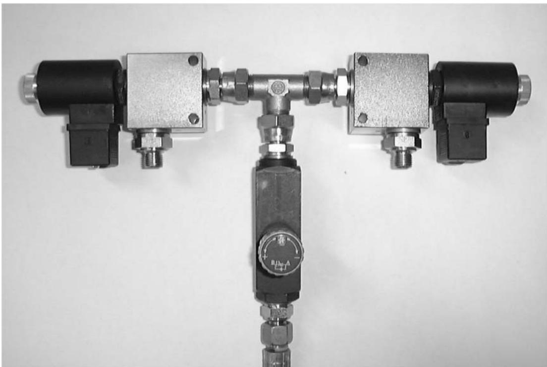
Fig. 7. The adjustable restrictor valve and two 2/2 directional valves with solenoids
