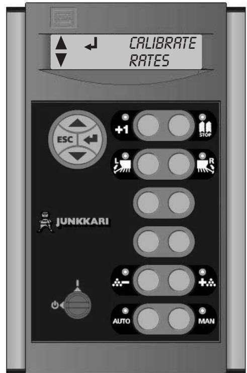
Turn the calibration test arm until the instrument beeps (0,012), -> enter the weight gained, enter it with arrow buttons. After confirming the weight gained with Enter button. The instrument will show " calibration complete".
