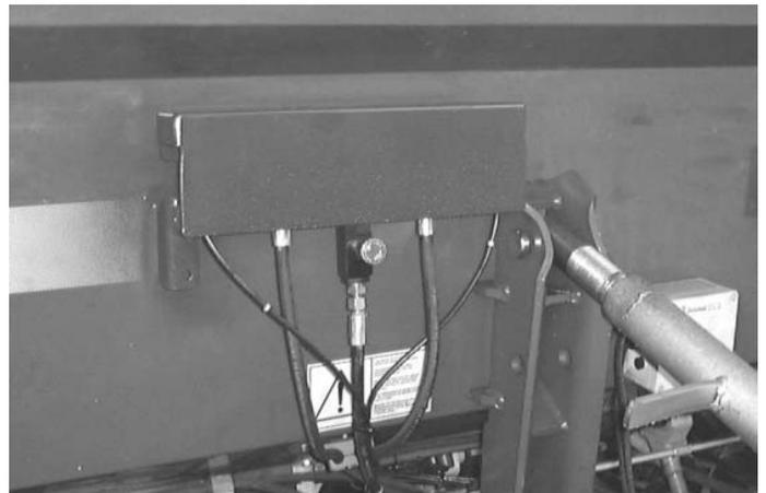
Fig.1. Placement of the valve pack and cover.
