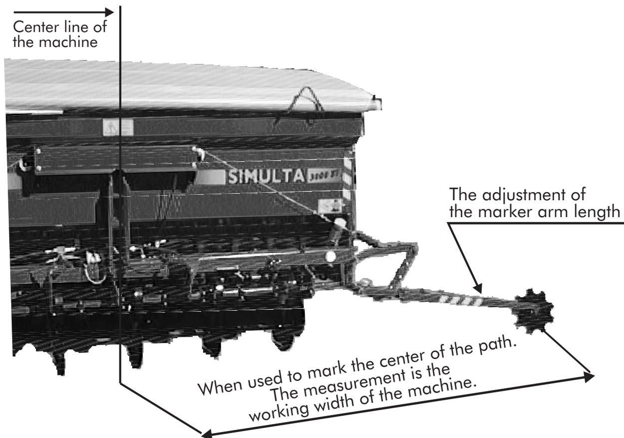
Fig. 5. The working width adjustment
