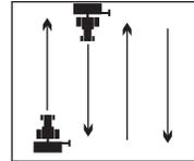
When the row marking is done to both sides of the drill, both markers are lowered down from the Expert.
