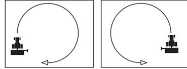
In the automatic row marking-mode the right and the left marker alternate, the change of side is done when the drill is lifted. Automatic operation can be started either left or right.
