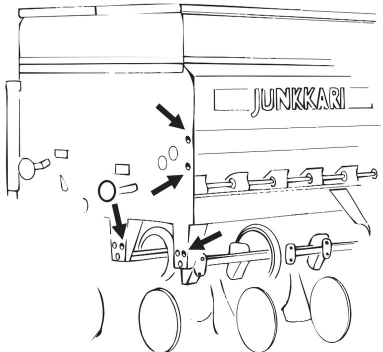
Fig. 2. Assembly holes for the turning unit at the side of the drill.
