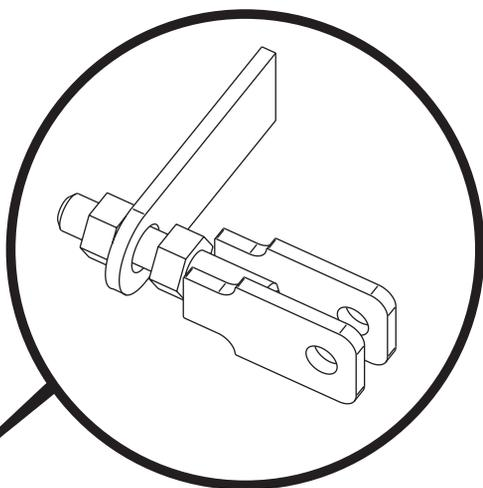
Adjust the hydraulic cylinder yoke to keep the marker resting against the cylinder when the it is in its shortest position, not against the turning unit. The linchpin is also then easy to remove. The yoke is locked after the adjustment by two nuts to the position where the hydraulic connection is upwards. (see fig. 3)
