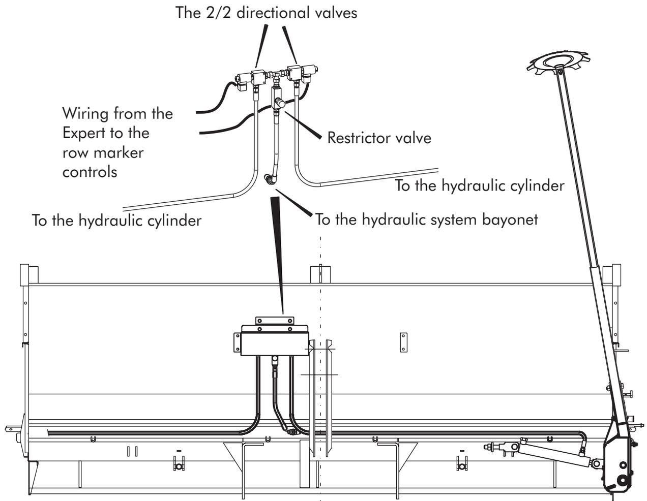
Fig. 4. The assembly of the row marker hydraulics to the seed and fertilizer drill
