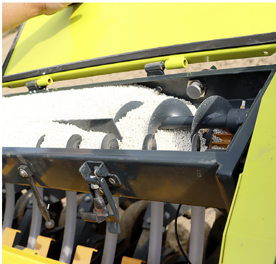
In driving direction, the rear augers fill one side of the metering units. The front augers return any excess material back into the system. As the wing hoppers start to empty, more material flows down from the main hopper through drop pipes, keeping the wing hoppers constantly filled. Each wing hopper has a sensor that alerts the operator on the screen when it runs empty. Before starting seeding, the wing hoppers are filled using a hydraulic motor.
