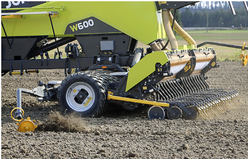
JUNKKARI'S DOUBLE disc coulters is suitable for ploughed, harrowed, and lightly tilled fields. Direct seeding is possible on lighter soils. The working depth is adjusted using a depth wheel for each coulter. Fine-tuning is done by raising or lowering the tractor's linkage, to which the drawbar is attached. The track marker folds to the rear.
