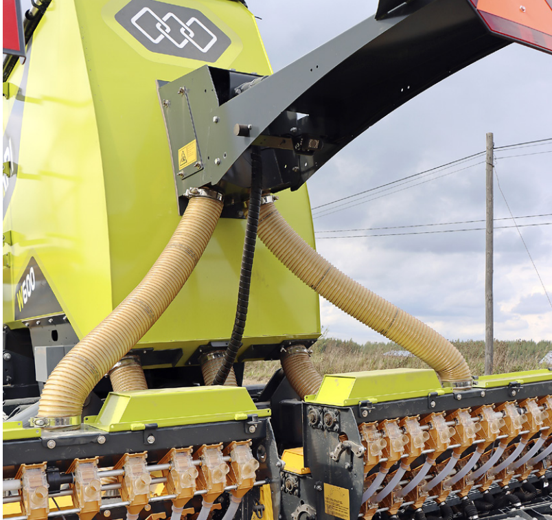
AN AUGER located at the bottom of the fertiliser hopper transfers the fertiliser into a “distribution box” at the rear of the hopper. From there, the material flows through pipes to the side sections. Gravity takes care of filling the side hoppers—as long as there is enough material in the main hopper.
