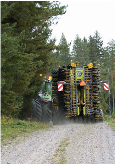
Although the centre of gravity in the Junkkari is relatively high, the machine remains stable during transport. On the road, the W600 runs on 12 centre-mounted packer wheels. These are divided into two bogie-type units with six wheels each, which pivot sideways and are mounted on a longitudinal axle. This design ensures that the outermost wheels also stay in contact with the ground, even if the middle of the road is higher than the edges.
